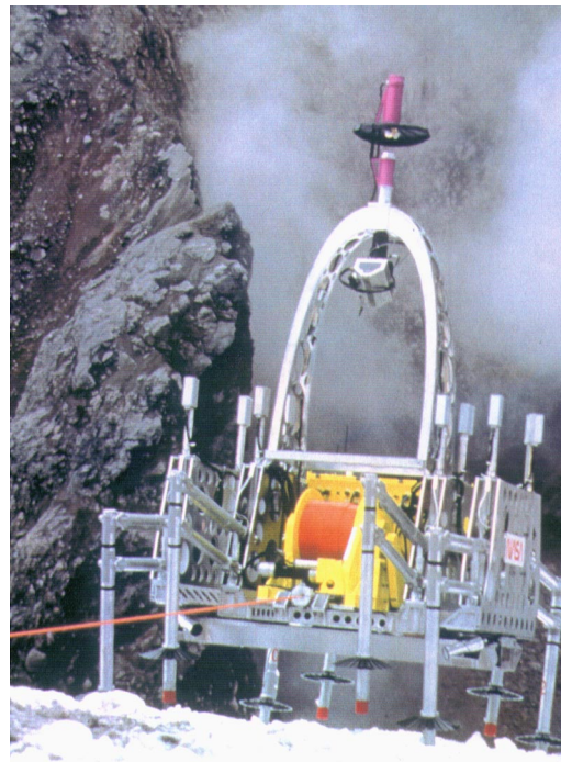
Figure 1: Dante II descending into the crater of Mount Spurr. then greater efficiency.
