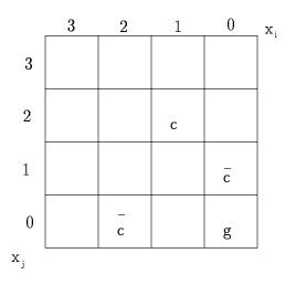
Figure 35: DIP 3  $c(x_i, x_j) = \overline{x}_i x_j, \ \overline{c} = x_i + \overline{x}_j$
