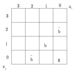
Figure 34: DIP 2  $b(x_i, x_j) = \overline{x}_i \overline{x}_j, \ \overline{b} = x_i + x_j$
