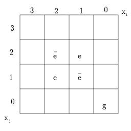
Figure 37: DIP 5  $d(x_i, x_j) = x_i \oplus x_j, \ \overline{d} = x_i \odot x_j$
