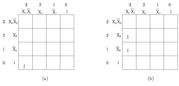
Figure 28:  $F(x_1, x_2) = x_1 \overline{x}_1, F(x_1, x_2) = x_1 \overline{x}_1 x_2 + x_1 \overline{x}_1 \overline{x}_2$
