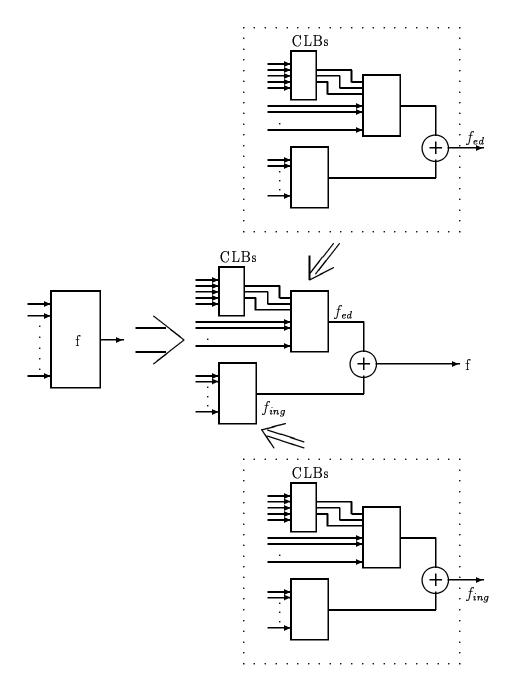
Figure 68: Application of local transformation to FPGA mapping
