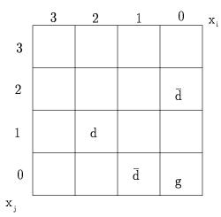
Figure 36: DIP 4  $d(x_i, x_j) = x_i \overline{x}_j, \ \overline{d} = \overline{x}_i + x_j$
