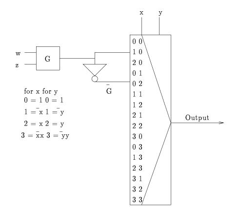
Figure 31: A Decomposition of a Fuzzy Function from Example 19.5 using a Fuzzy Multiplexer.
