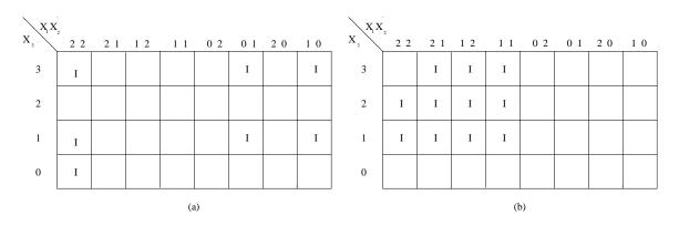
Figure 38: Illustration of compatible columns for a Fuzzy function
