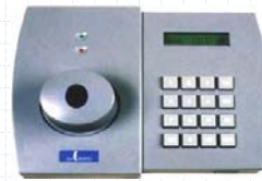
Retinal recognition system [Icam 2001 by Eyedentify]
