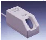
Optical fingerprint sensor [Fingerprint Identification Unit FIU-001/500 by Sony]
