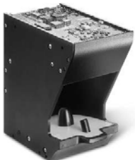
Hand geometry reader for two finger recognition by BioMet Partners
