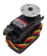
position control. The motors inside the servo only hold position when powered so when the power is removed any weight bearing servos release. The wrist on the robot is an example of this. When the program is running the wrist servo supports the hand, but as soon as power is removed or the program is ended the hand falls to one of the servo extremes.
