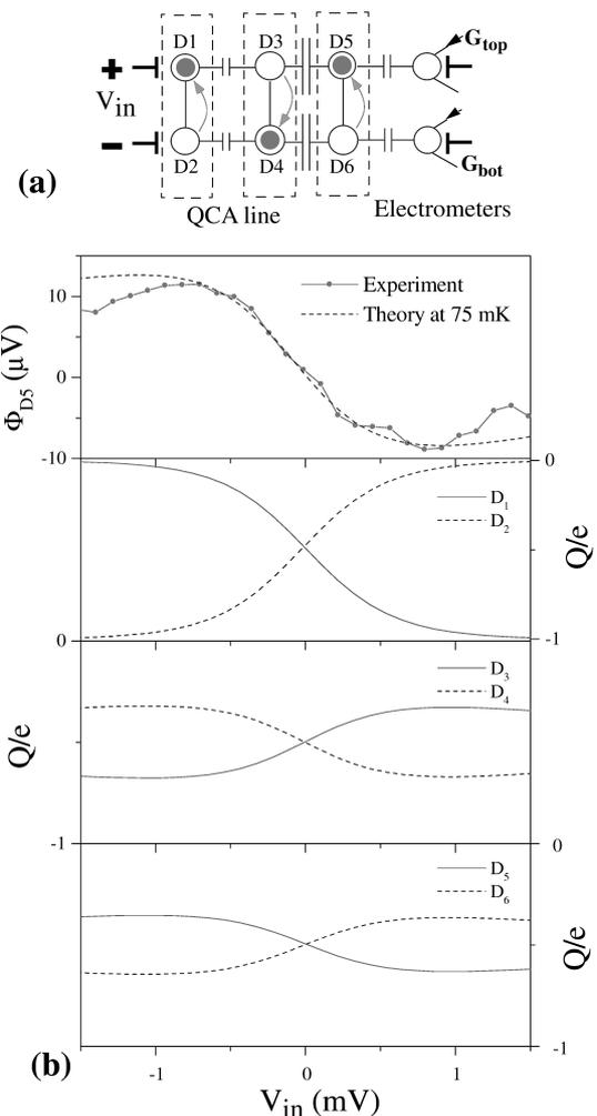
Fig. 4. (a) Simplified schematic of the three cell line using two-dot QCA. (b) Experimental and theoretical data showing the operation of the line. Top panel shows the potential on dot D5, and the lower three panels show the charge on the dots within each cell.
