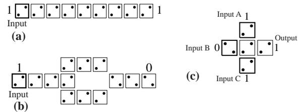
Fig. 2. (a) Line of QCA cells. (b) QCA inverter. (c) QCA majority gate.
