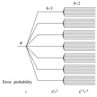
Figure 7. Concatenation of the seven-bit code. If the error rate is  $\epsilon$  for the qubits, the encoding will gives a rate of  $C^{2^h-1}\epsilon^{2^h}$  for the hth level of the hierarchy.
