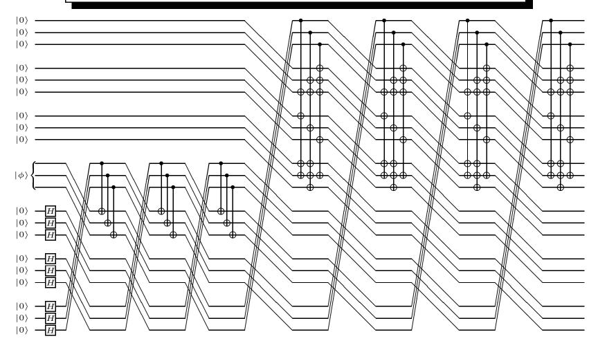
Encoder for the quantum Reed-Solomon code [[21,3,5]] using quantum shift registers for the multiplication by  $\tilde{\boldsymbol{g}}(X) = X+1$  and  $\boldsymbol{g}^{\perp} = \alpha X^3 + X^2 + \alpha^2 X + 1$ .
