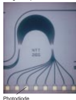
8-channel demultiplexer with integrated photo-detectors
