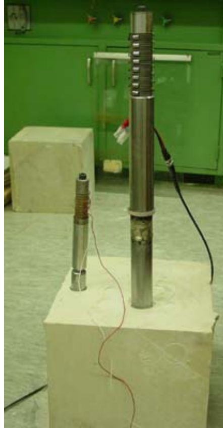
Ultrasonic Gophers for deep drilling
