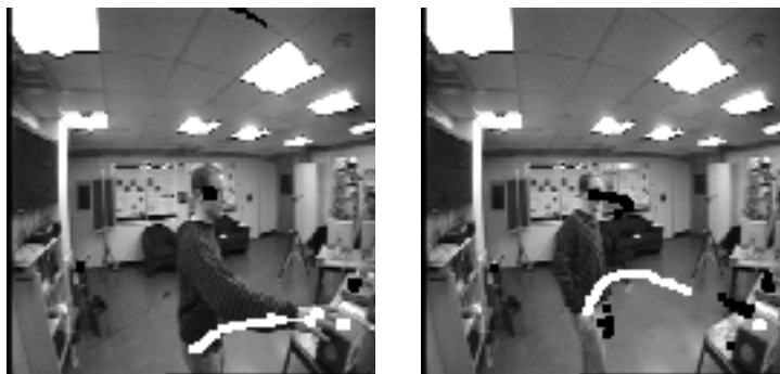
Figure 11-1: The intentionality detector seeks to label the intentional relationships for basic approach and withdrawal. The image at left shows a person reaching for a toy block with the trajectory positions drawn on the image. This trajectory was classified as an approach event. At right, an event that was classified as a withdrawal event when the person then quickly pulled his hand away.
