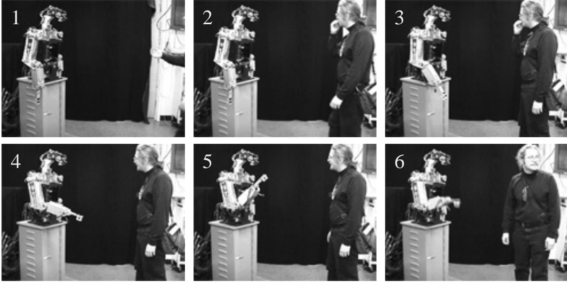
Figure 9-4: Cog mimicking a person making the American Sign Language sign for food. The person began making the gesture before entering the field of view of the video camera, but the length of time of each gesture was still similar.
