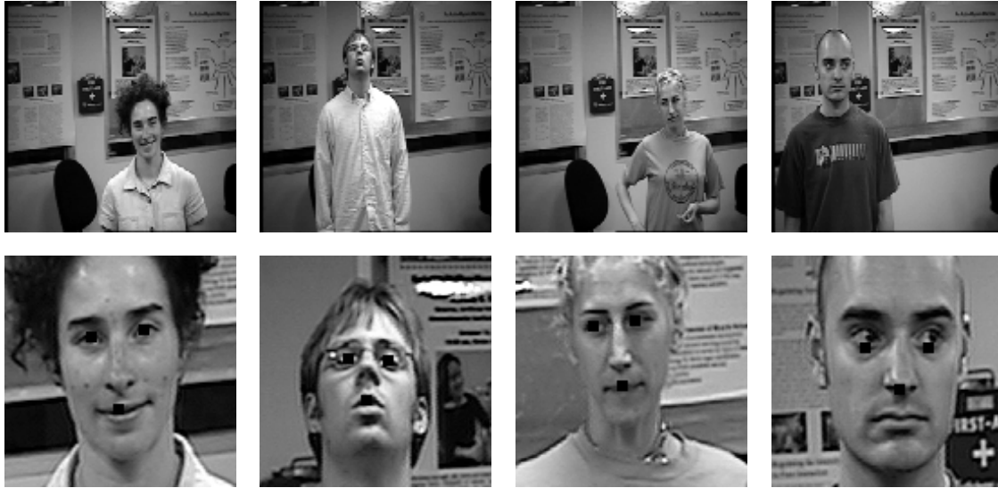
Figure 8-5: Eye and mouth regions detected by the multi-stage classifier system from figure 8-1. The top row contains the foveal images acquired immediately after a saccade, while the lower row contains the result of the feature identification system. The positions of the eyes and the mouth are shown with black dots. The first three cases were successful, but the last examples failed due to a mis-match of the feature set to the nostrils rather than the mouth.
