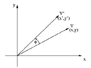
Rotation of a vector V by the angle  $\phi$ The individual equations for x' and y' can be rewritten as:
