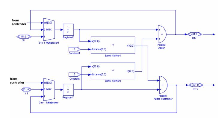
2.3 RTL Schematic of the Cordic-HT Cell:
