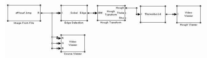
Here we see that an image from the file is passed to a Sobel edge detector block which transforms the image into a binary image with color white representing edges. Then the standard Hough transform of the edge detected image is performed, which outputs a space matrix of rho and theta values. The threshold block finds peaks in the space matrix which then corresponds to the lines or any arbitrary shapes of the feature in the original image.
