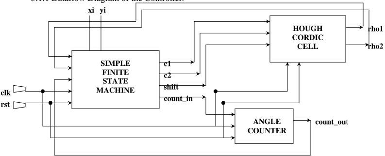
5.1.1 Dataflow Diagram of the Controller:
