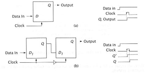
Figure 2.2 Edge-triggered clocks. (a) Single rank. (b) Dual rank.
