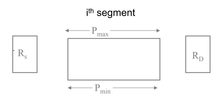
At time =  $t_1$  let data<sub>1</sub> proceed into pipeline stage It can be safely clocked at the destination latch at time  $t_3$  $t_3 = t_1 + P_{max} + C$ But new data<sub>2</sub> can proceed into the pipeline earlier by an amount  $P_{min}$ say, at time  $t_2$ , where  $t_2 = t_1 + P_{max} + C - P_{min}$  so that
