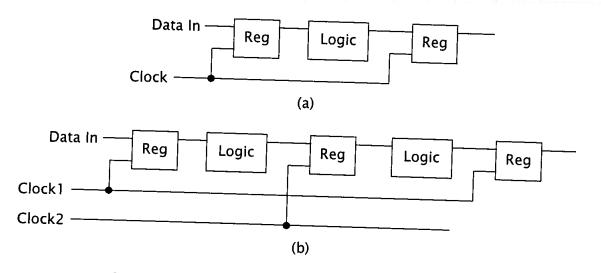
Figure 2.5 Clocks. (a) Single phase. (b) Two-phase.
