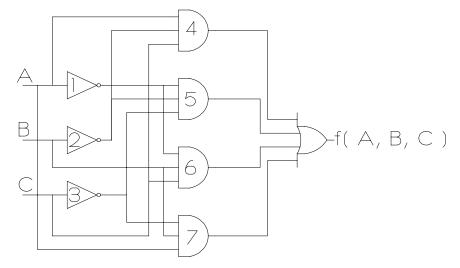
$f_{odd}(A,B,C) = A\overline{B}C + \overline{A}\overline{B}\overline{C} + \overline{A}BC + AB\overline{C}$
