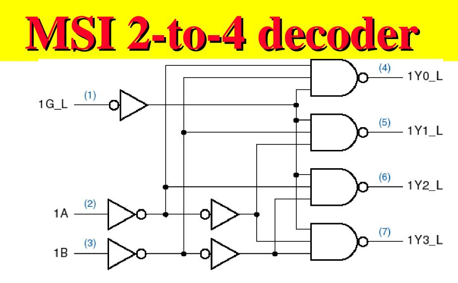
Input buffering (less load)NAND gates (faster)
