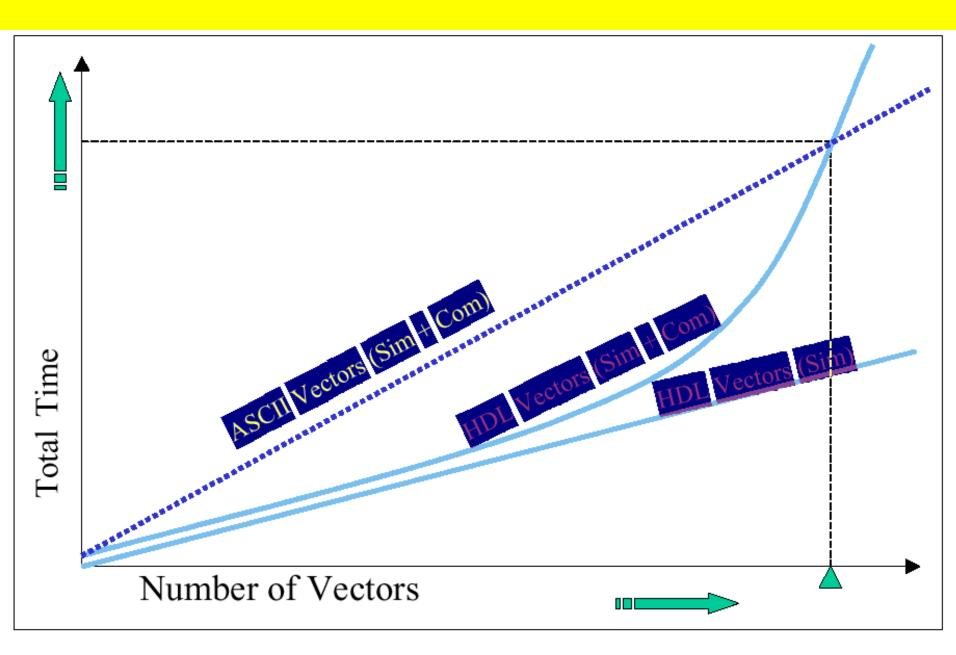
Figure 1: Vectors in ASCII vs. Vectors in VHDL
