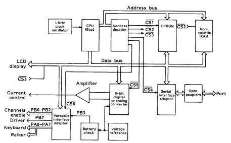
Figure 2 Block diagram of the stimulator microboard
