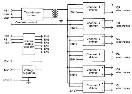
Figure 3 Block diagram of the stimulator driver board
