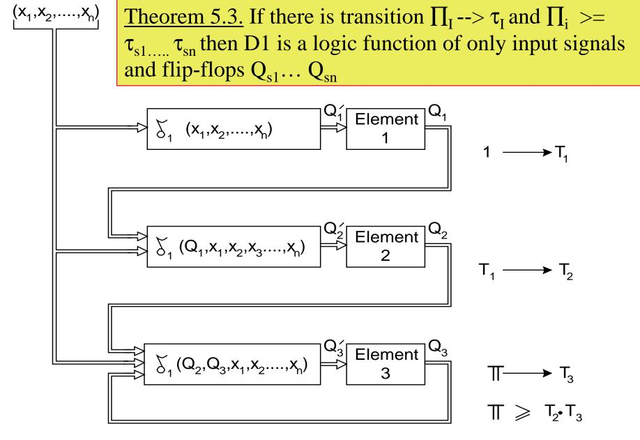
Fig.5.37. Structure of automaton illustrating application of Theorem 5.3
