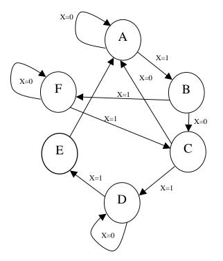
A 000 B 001 C 010 D 100 E 101 F 011 Q0 = XC + X'D + [XD]Q1 = X'B + XF + [X'F + XB]Q2 = XA + [XD] + [X'F + XB]
