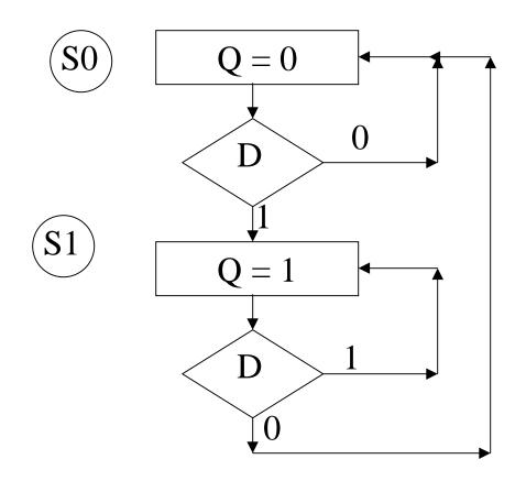
A Finite State Machine (FSM) can be described via either a Bubble diagram or an ASM chart.
