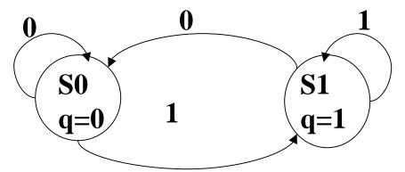
Bubble Diagram: States represented by bubbles. State transitions represented by arrows. Labeling on arrows represent input values (in this case, the D-input!). Labeling inside bubbles represent output values.
