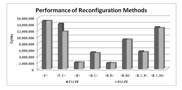
Fig. 4.4: Reconfiguration latencies using the notation in table 4.1.
