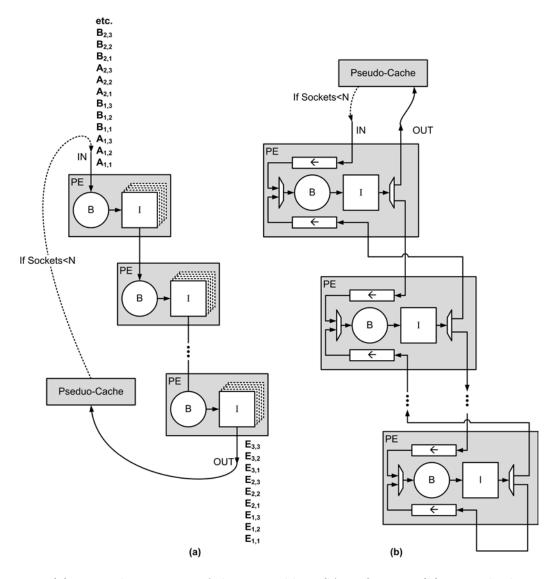
Fig. 3.7: (a) Vertical projection of the 2D Faddeev SA in fig. 3.6. (b) Looped adaptation of fig. 3.7(a). B=Boundary Cell, I=Internal Cell.
