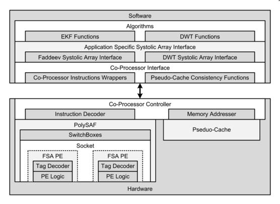
Fig. 3.2: This figure shows the software interface abstraction layers and the hardware interfaces within the co-processor for implementing the EKF and DWT algorithms.
