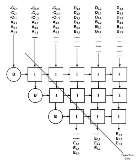
Fig. 3.6: 2D direct mapping of the Faddeev systolic array. B=Boundary Cell, I=Internal Cell.
