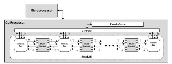
Fig. 3.1: This figure shows the system architecture with details on the PolySAF.
