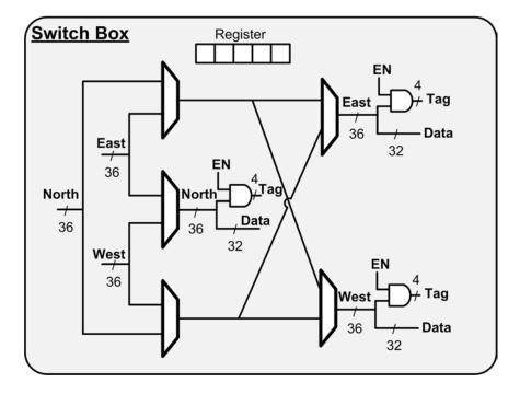
Fig. 3.3: This figure shows the internal structure of a switchbox.
