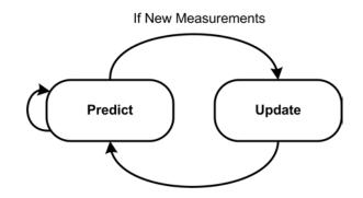
Fig. 2.1: Kalman filter process cycle.
