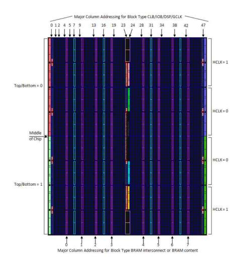
Fig. 2.3: Configuration layout of the Virtex 4 FPGA.
