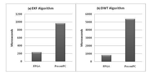
Fig. 4.3: (a)Comparison of the EKF run the FPGA and PowerPC for the test case defined by Ronnback [11]. (b) Comparison of the DWT run on the PowerPC for a test case of a 64x64 image and 4 taps.
