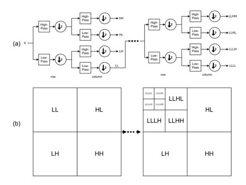
Fig. 2.2: (a) 2D DWT algorithm. (b) Image partitioning after three decomposition levels. L=Low-pass. H=High-pass.
