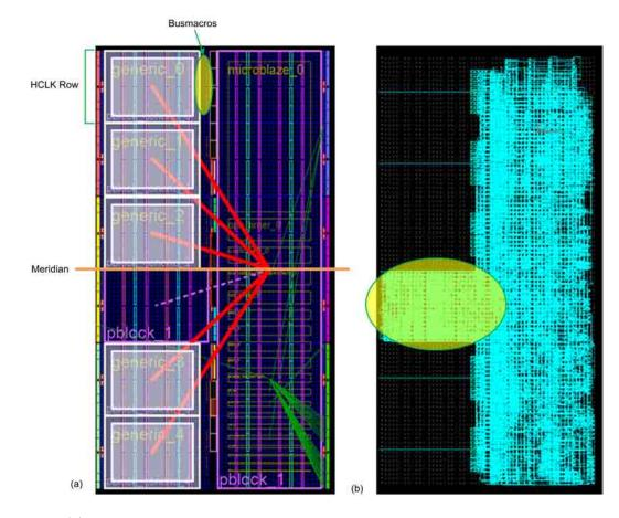
Fig. 4.1: (a) Shows the design floorplanned with the sockets highlighted in white, and the busmacros circled in yellow. (b) The the routed static design.
