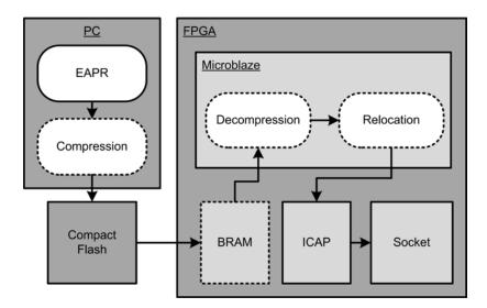
Fig. 3.10: This figure shows the data flow of a partial bitstream in the Hybrid PDR method. Dotted boxes represent optional stages.
