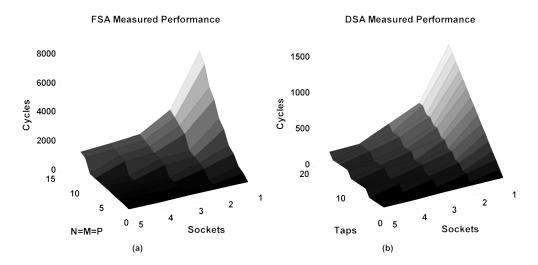
Fig. 4.2: (a) Trade-off between size of the input (1 to 16) number of sockets (1 to 5) for the FSA. (b) Trade-off between the number of filter taps (1 to 16) number of sockets (1 to 5) for in an input vector of 16 on the DSA.
