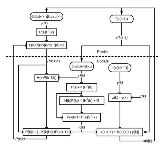
Fig. 3.5: This figures shows the mapping of the EKF onto the Faddeev algorithm. Rounded boxes represent operations performed in software on the microprocessor, and squared boxes represent operations performed by the a the hardware accelerator.
