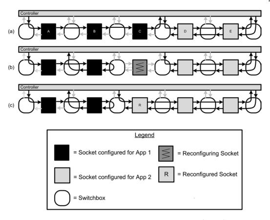
Fig. 3.4: This figures shows an example of scaling down one SA (App 1) and scaling up another SA (App 2).
