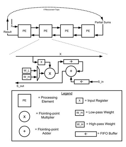
Fig. 3.9: DSA internal structure.
