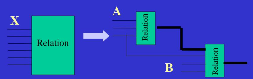
if  $A \cap B = \emptyset$ , it is disjoint decomposition if  $A \cap B \neq \emptyset$ , it is non-disjoint decomposition
