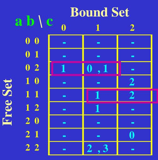
Columns 0 and 1 and columns 0 and 2 are compatible column compatibility index = 2
