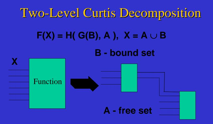
if  $A \cap B = \emptyset$ , it is disjoint decomposition if  $A \cap B \neq \emptyset$ , it is non-disjoint decomposition
