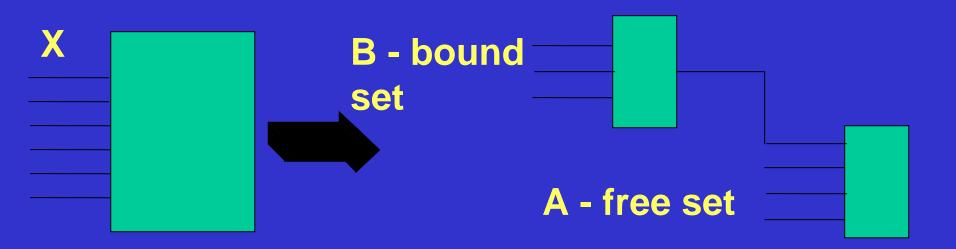
if  $A \cap B = \emptyset$ , it is disjoint decomposition if  $A \cap B \neq \emptyset$ , it is non-disjoint decomposition
