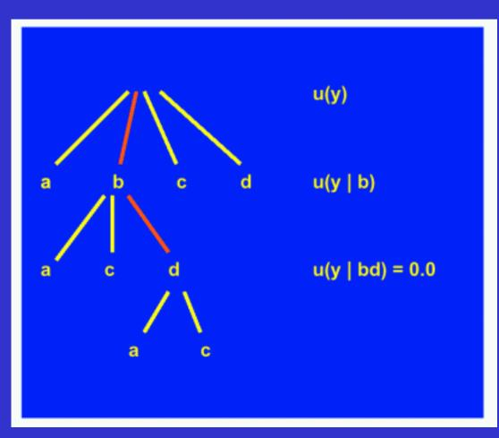
Variables b and d reduce uncertainty of y to 0 which means they provide all the information necessary for determination of the output y
